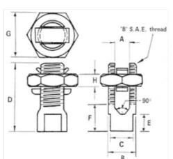
**Bervic Split Bolt Clamps** are made of 100% Australian Brass and comes in a plain or electro-tinned finish.
