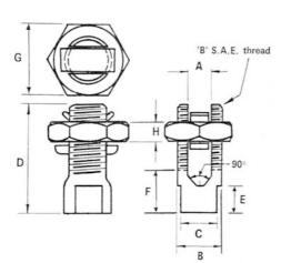
**Bervic Split Bolt Clamps** are made of 100% Australian Brass and comes in a plain or electro-tinned finish.
